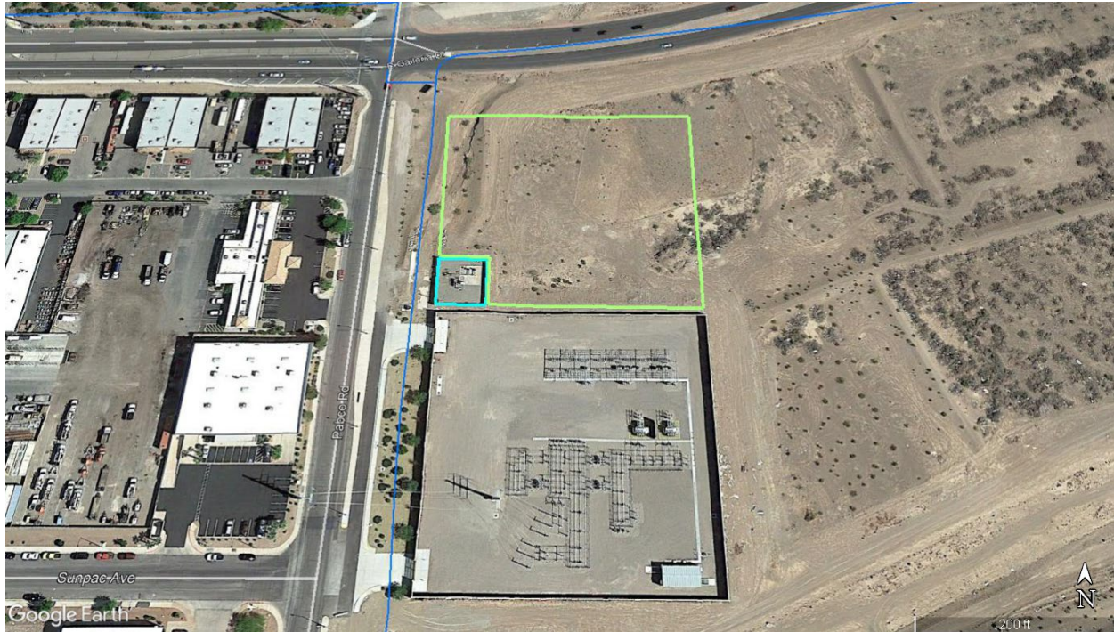
Depiction of the area needed for solar PV located immediately north of LS-2 (green outline) assuming baseline plus 100% usage increase (2.2 Acres). LS-2 is outlined in blue (0.1 Acres). Shown only for the purpose of demonstrating scale, not for construction.
