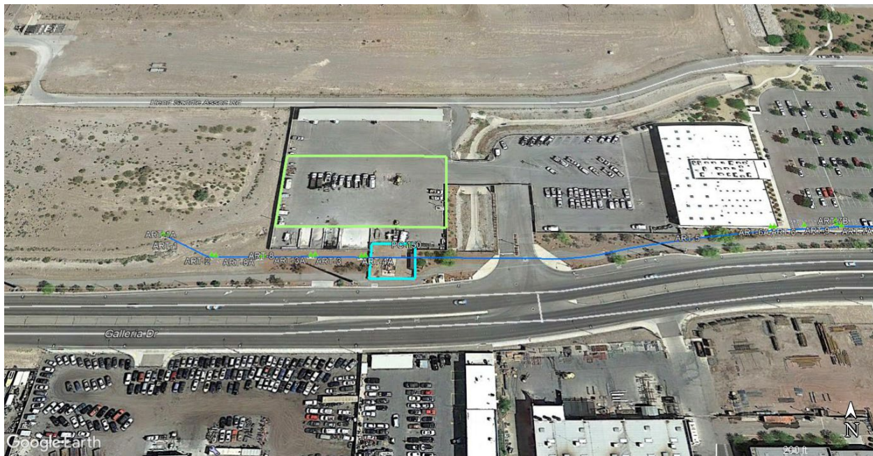
Depiction of the area needed for solar PV located immediately north of LS-3 (green outline) assuming baseline plus 100% usage increase (0.80 Acres). LS-3 is outlined in blue (0.1 Acres). Shown only for the purpose of demonstrating scale, not for construction.
