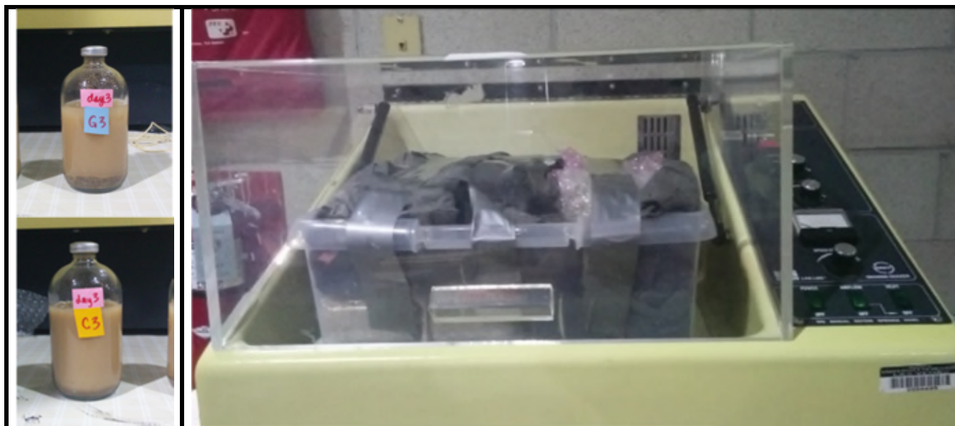
Figure 4: Microcosm bottles with vadose zone soils and SLMW (images on left) and incubation of bottles in a horizontal mixing shaker covered with felt to avoid light exposure and potential algae growth (image on right).
