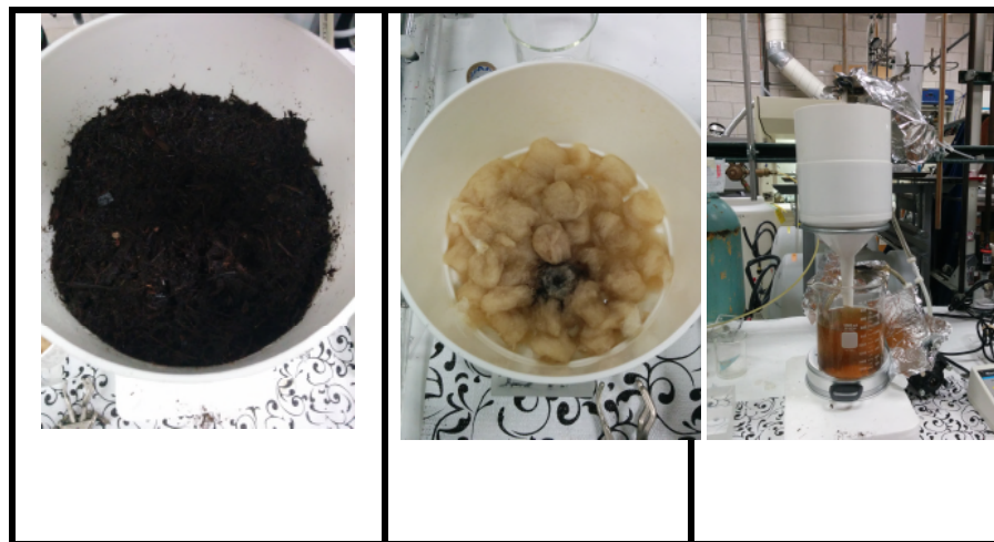
Figure 2: Compost extract generation using compost in the bottom container and cotton balls in the top container.
