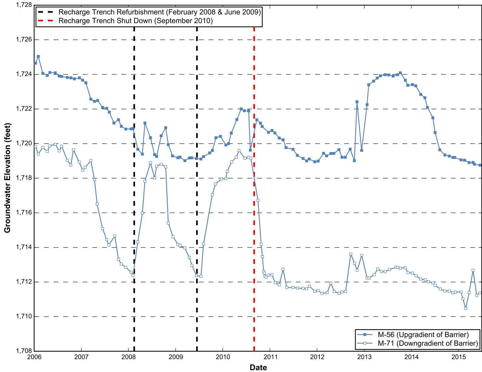
Hydrograph Pair Across the Barrier Wall - M-71 and M-56 Nevada Environmental Response Trust Site Henderson, Nevada
