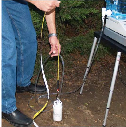
Fig. 18. Lowering RU and APM in borehole. Note do not hang from Tubing.
