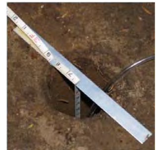
Fig. 19. Tape secured using Tape Holder.
