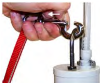
Fig. 15. Connecting Tape Hook to RU.
