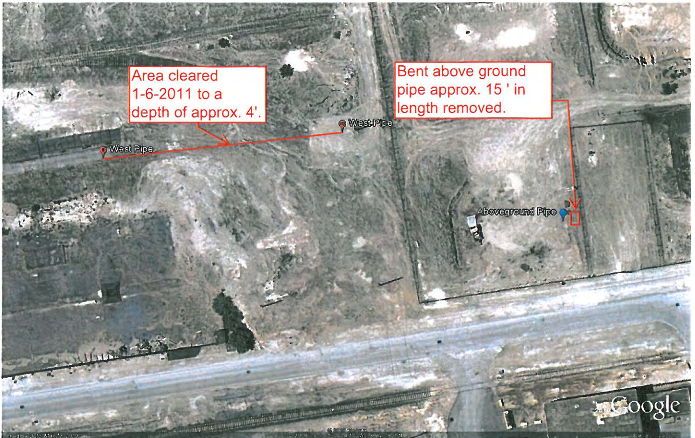
Tronox - 560 West Lake Mead Pkwy. Henderson NV 1-06-2011 Red line indicates area that was cleared for 20" transite and asbestos wrapped steel pipe 10" and 8" diameter by Converse Consultants to a depth of approximately four feet. Red box area was also cleared. Approximately 15 feet of 8" asbestos wrapped steel pipe had been protruding above ground in the area indicated by the red rectangle.
