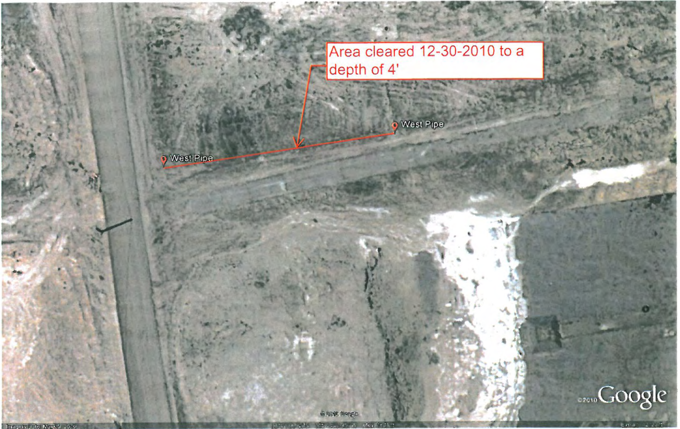
Tronox - 560 West Lake Mead Pkwy. Henderson NV 12-30-2010 Red line indicates area that was cleared for 20" transite and asbestos wrapped steel pipe 10" and 8" diameter by Converse Consultants to a depth of approximately four feet.
