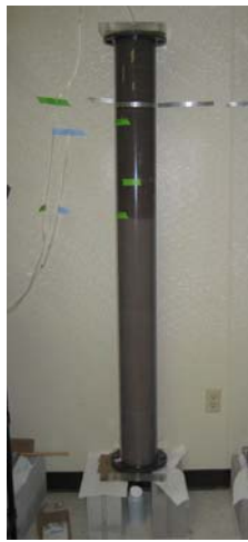
Figure 6. Soil Flush Column near Beginning of Test.
