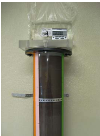
Figure 5. Addition of Water via Gravity Feed into Percolation Column. Note: wetting front below silver band.
