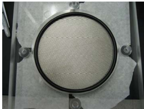
Figure 2. Bottom endplate with stainless steel disk and o-ring.
