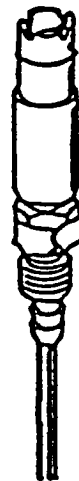
PVC Bottom Emptying Device with tap. Use in the Acrylic and PVC bails. This model has the metal push clip on it for flow control.
