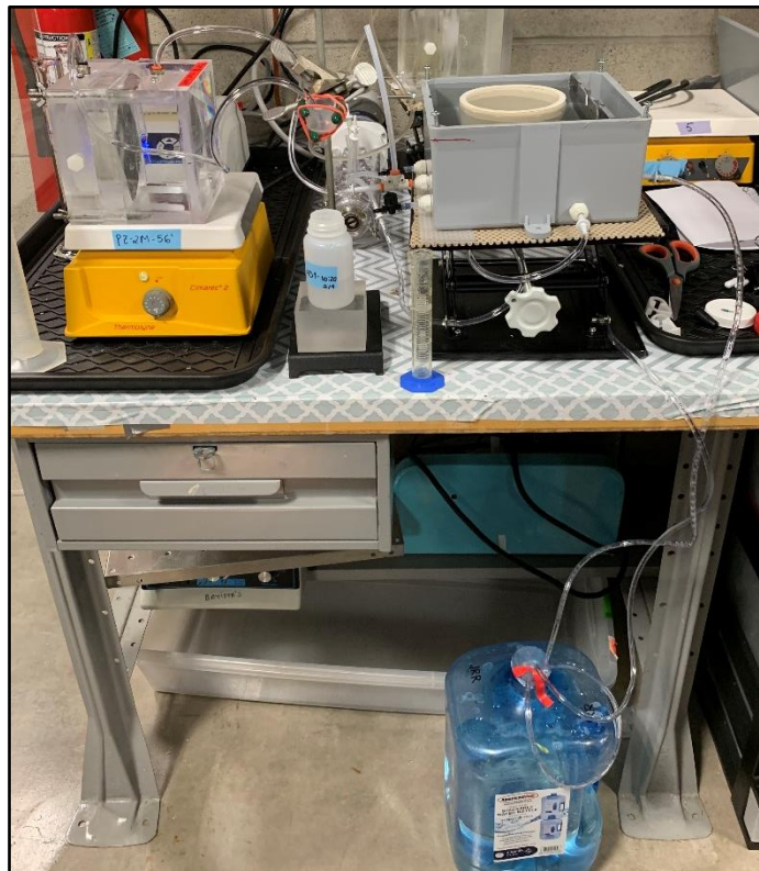
Figure 27 – Final advection test setup using the stable water level box connected to the chamber's arrangement.
