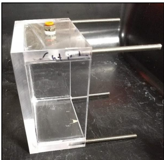
Figure 10 - Tracer solution chamber built in acrylic with four long screws to hold the other parts of the set up together.
