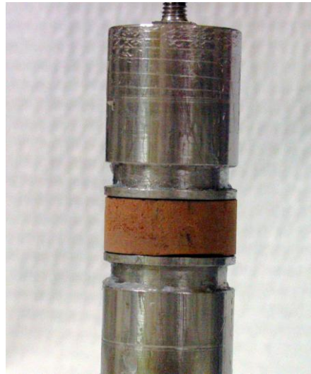
Figure 16: Rock Core Sample (shale) Enclosed by End Pieces to be Used in a Permeability Measurement
