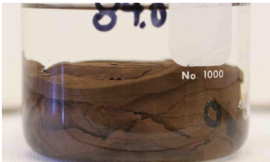
Figure 23: Core Slice of Queenston Shale Immersed in 170 g/L KNO 3 Showing a Parting Pattern Typical of Unconfined Samples Immersed in Water
