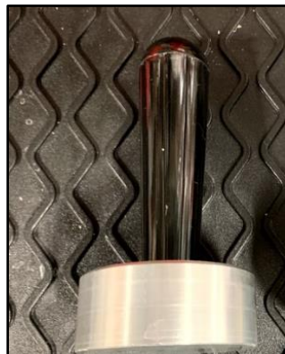
Figure 1 - Soil weight pusher with 2.4 inches diameter used to extrude samples from the small California Tubes.
