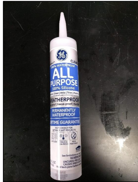
Figure 19 – Specifications of the silicone glue used to attach the soil to the acrylic block.
