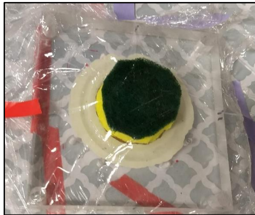
Figure 24 – Soil sample attached to the support protected by the damp sponge and wrapped in a plastic film during the drying period.
