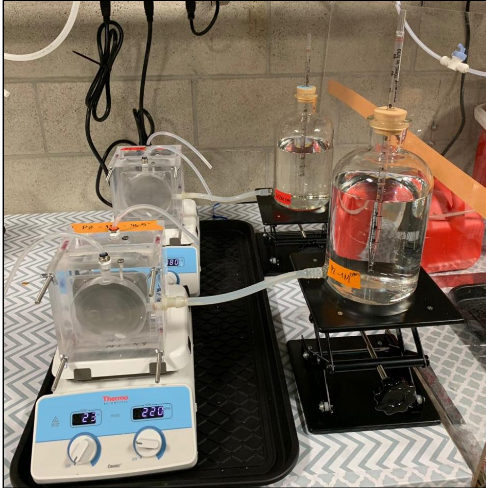
Figure 17 – Final diffusion chamber setup for the diffusion test, using a Mariotte Bottle to fill the eluent reservoir.
