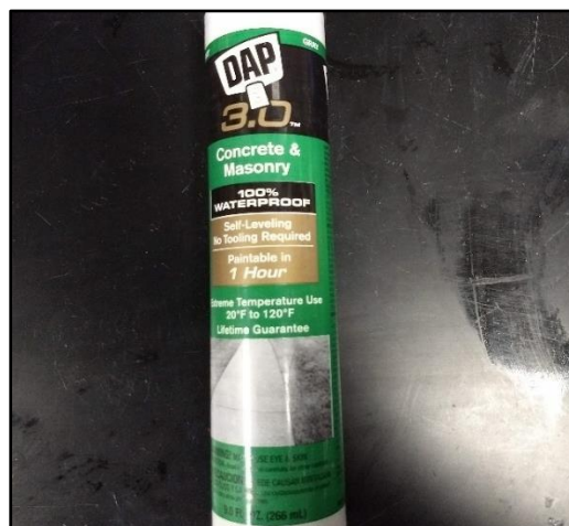
Figure 22 – Specifications of the concrete & masonry adhesive used to attach the soil samples to the diffusion chamber.
