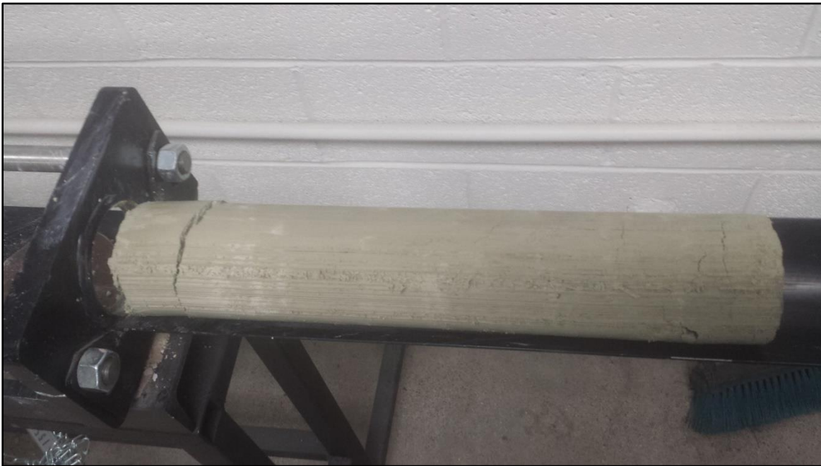
Figure 2 - Extracted 30-inch core sample after extrusion with the California Tube extrusion apparatus.
