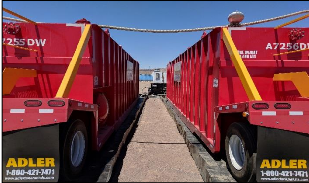
3. Double-wall frac tank setup
