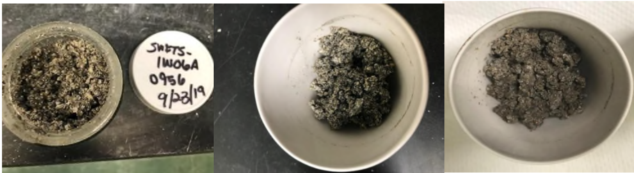
Fig. 3. IW-06A Precipitate pictures before heating, after heating, and after volatilization (left to right)
