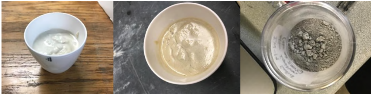
Fig. 1. IW-19 Precipitate pictures before heating, after heating, and after volatilization (left to right)
