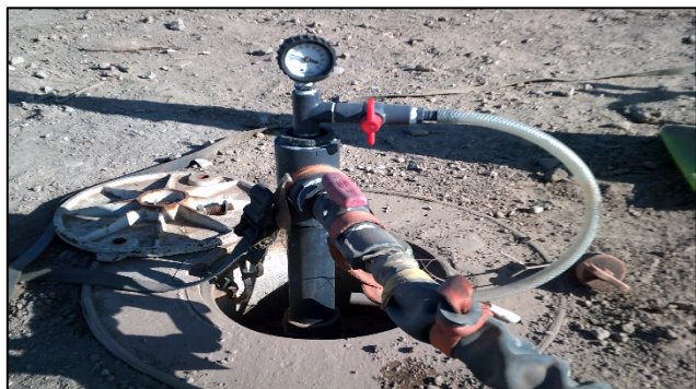
16. Well head adapter, complete with pressure relief valve and pressure gauge (60 PSI)
