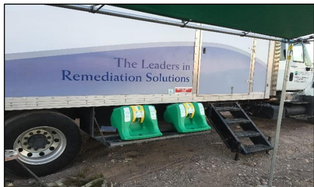
7. Emergency Eye Wash Station
