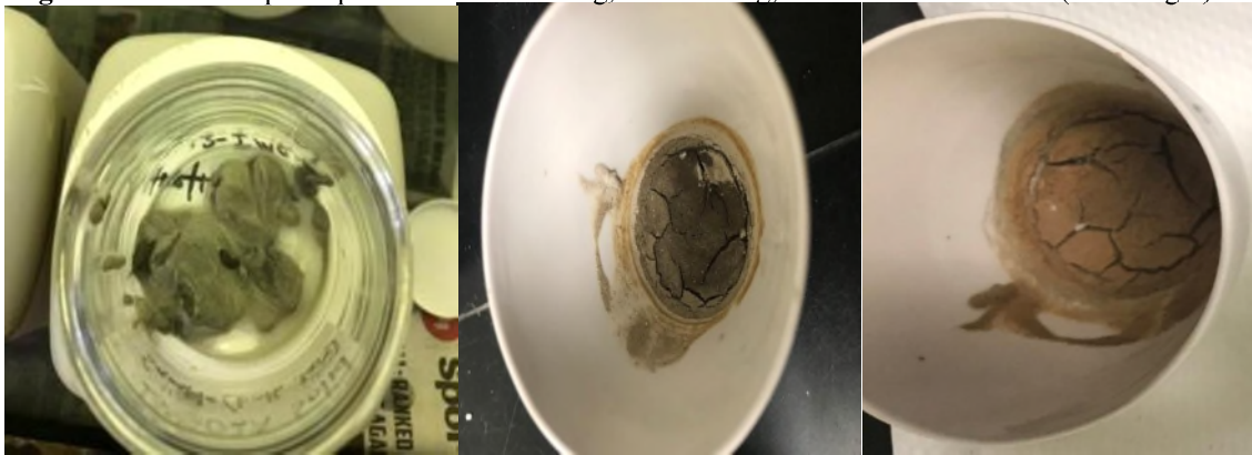
Fig. 4. IW-02A Precipitate pictures before heating, after heating, and after volatilization (left to right)
