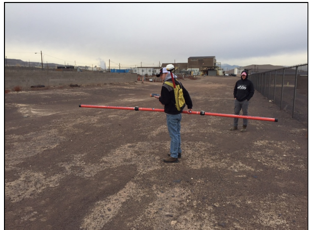
4 : EM31 Terrain Conductivity Meter with GPS
