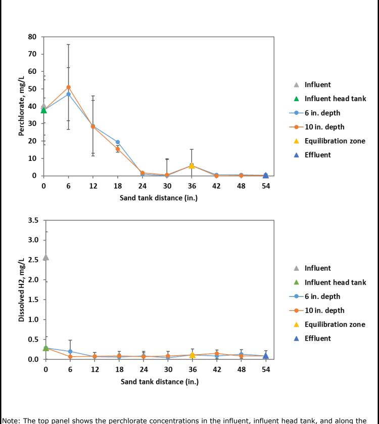
Note: The top panel shows the perchlorate concentrations in the influent, influent head tank, and along the sand tank flow path at depths of 6 inches (in.) and 10 in. The bottom panel shows dissolved hydrogen distribution in the influent, influent head tank, and along the sand tank flow path at depths of 6 in. and 10 in.
