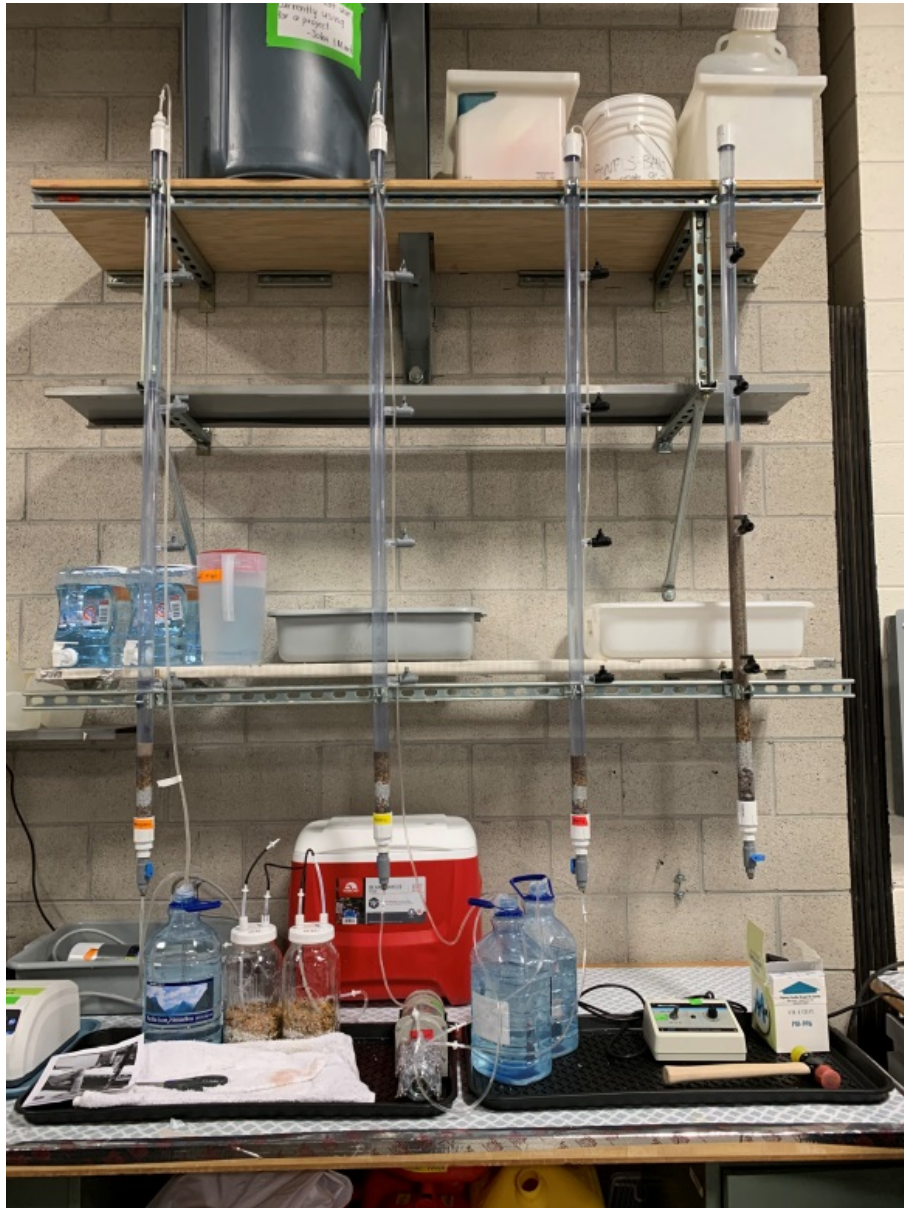
Photo 1. Flow-through column tests with site soils. Four new, longer columns (5 feet long) have been built with ports along the side. These columns will be used to determine degradation of varying concentrations of contaminants and also to measure head loss. One of these columns has been fitted differently to test the Peroxychem EHC, a commercially-available ZVI/organics mixture. The set up contains two settling bottles (left side of photo) to settle the fine material generated with the Peroxychem EHC.
