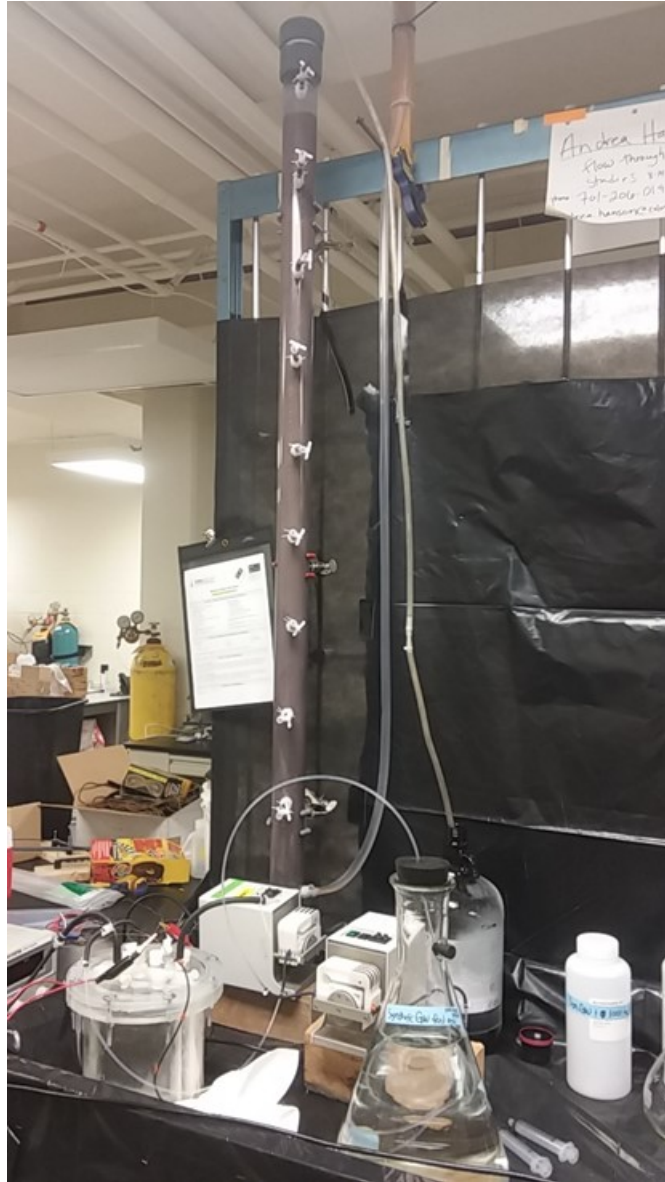
Photo 2: Experimental setup for flow-through column testing. This 2" diameter, 5' long PVC test column has equally-spaced sampling ports along the flow path, allowing the research team to obtain detailed information of perchlorate and other competing electron acceptor removal. Not visible in the figure are gas management system and biomass sampling ports on the back side of the column. This photo also shows an electrochemical reactor of the kind used in the batch study phase, in the lower left corner.
