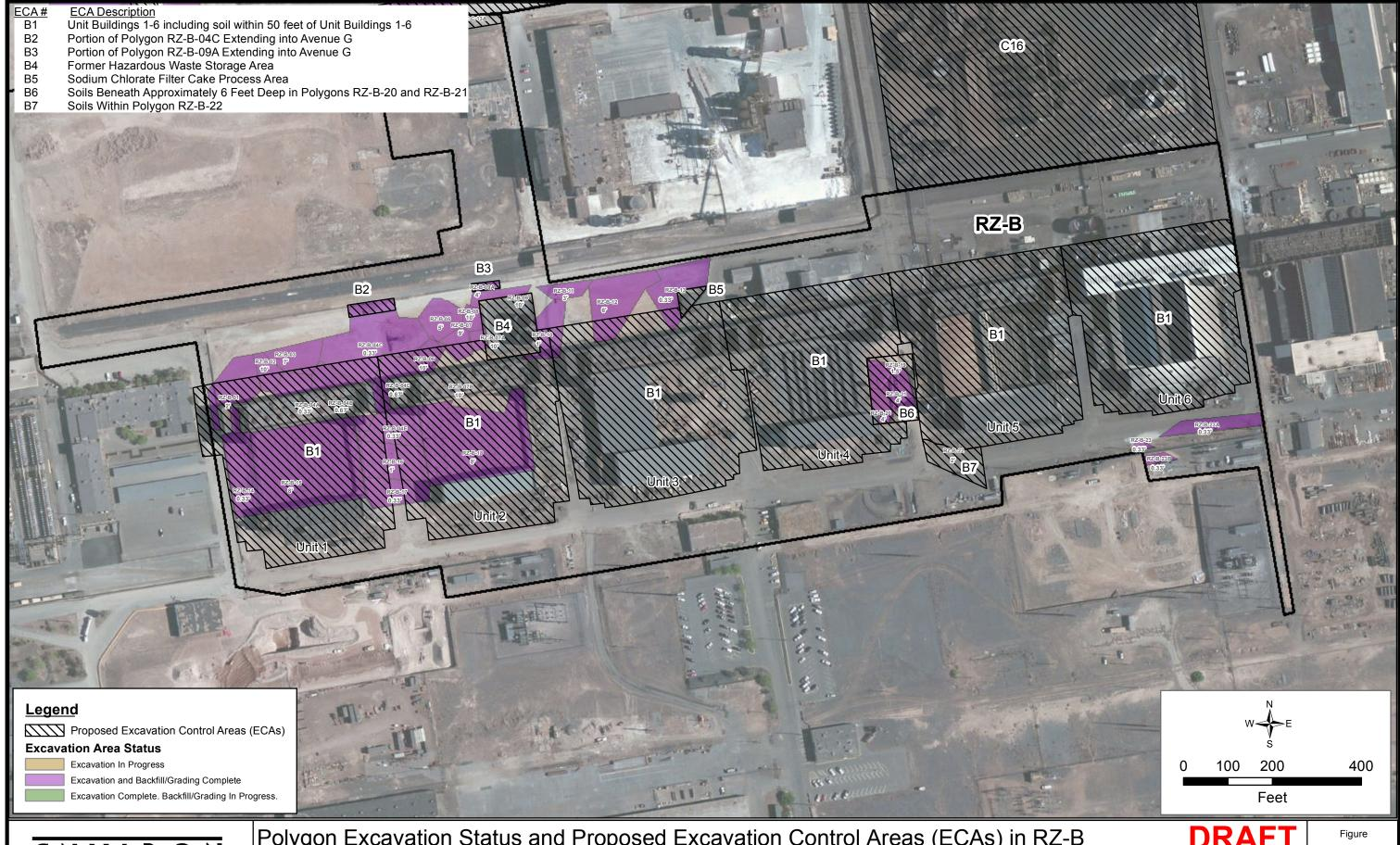
Polygon Excavation Status and Proposed Excavation Control Areas (ECAs) in RZ-B Nevada Environmental Response Trust Site, Henderson, Nevada
