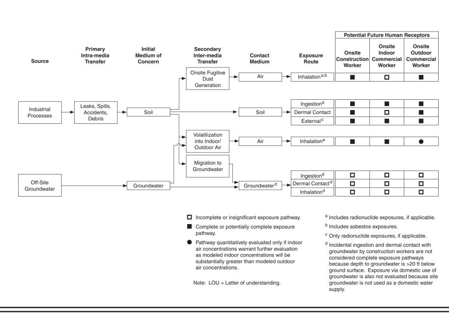
Figure 7. Conceptual site model diagram for potential human exposures—Parcels C, D, F, G, and H, Tronox Facility, Henderson, Nevada
