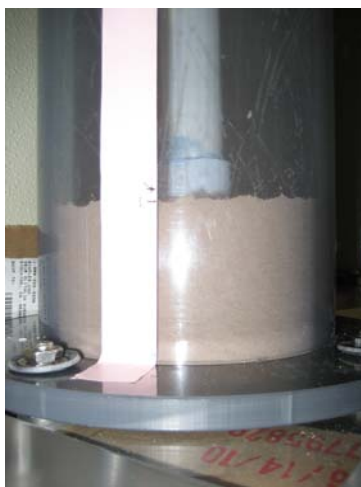
Figure 4. Addition of the first lift to a column.
