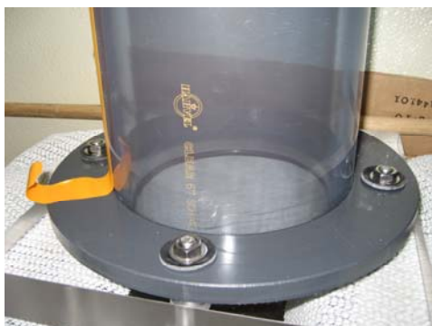
Figure 3. Column bolted to bottom endplate.
