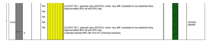
Project No. 3850360 Log of Boring: BRC-SB-19-A
