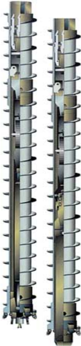
Figure 1 Typical Wireline Coring Devices
