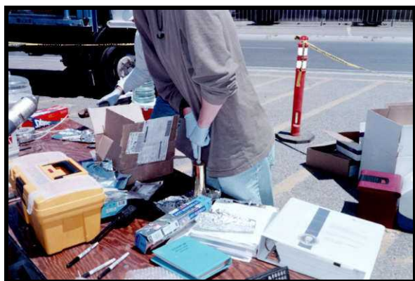
Figure 4a. Inserting EnCore™ Sampler into Soil
