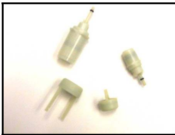
Figure 1b. EnCore™ Samplers, 5-gram and 25-gram
