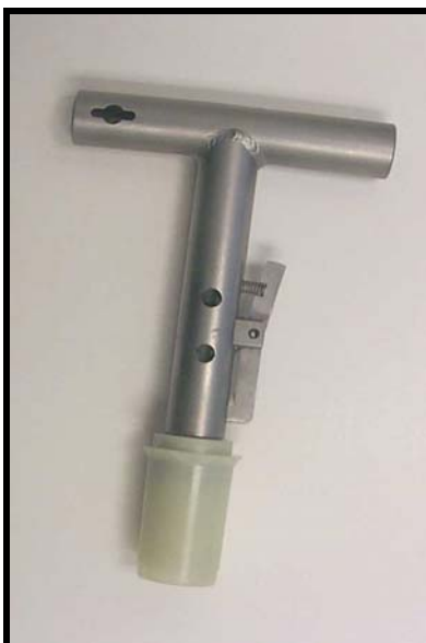
Figure 3. T-Handle and Sampler in Locked Position
