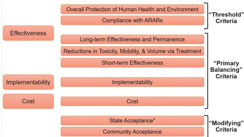
Figure 4: Identification of the nine evaluation criteria and their role in remedial alternative evaluation and comparison
