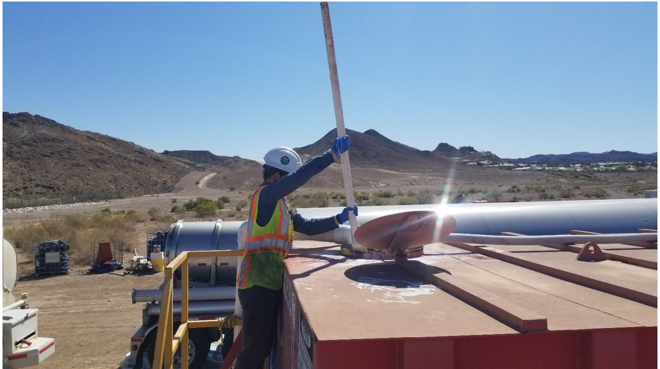
Collecting a sample of the injectate solution for specific gravity analysis to ensure the solution is mixed thoroughly prior to injection.
