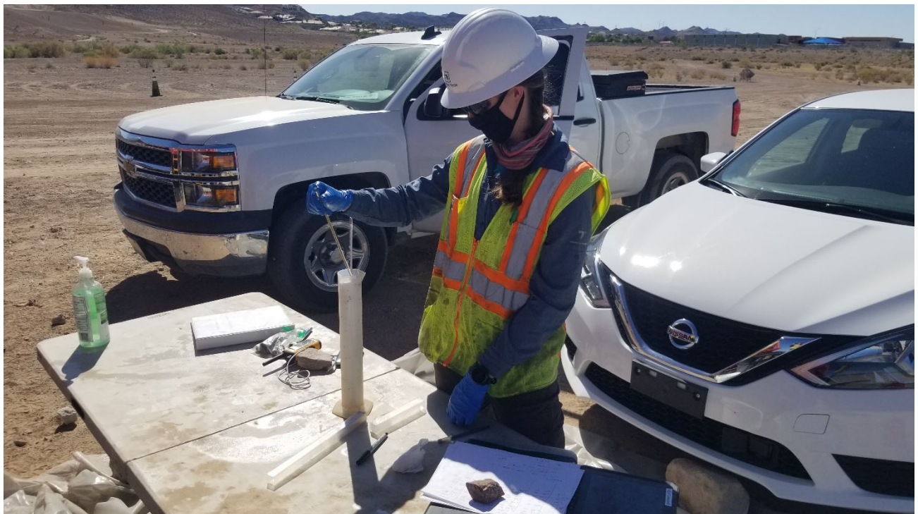
Measuring specific gravity and temperature of injectate solution sample.
