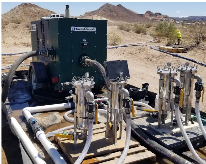
Right: Four bag filters are used to filter sediment from the extracted groundwater prior to the groundwater being pumped to the frac tanks/injection system in the laydown area. Left: Extraction manifold with flow meter for each extraction well.
