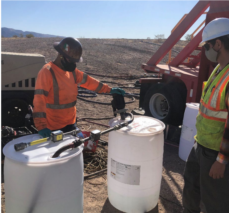
Left: Testing and calibrating flow meters; Right: Tested flow meters
