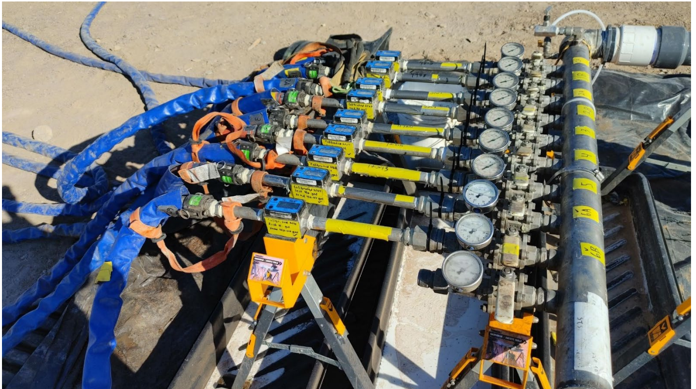
Manifold A with Calibrated Flow Meters, Pressure Gauges, and Well Connection Labels
