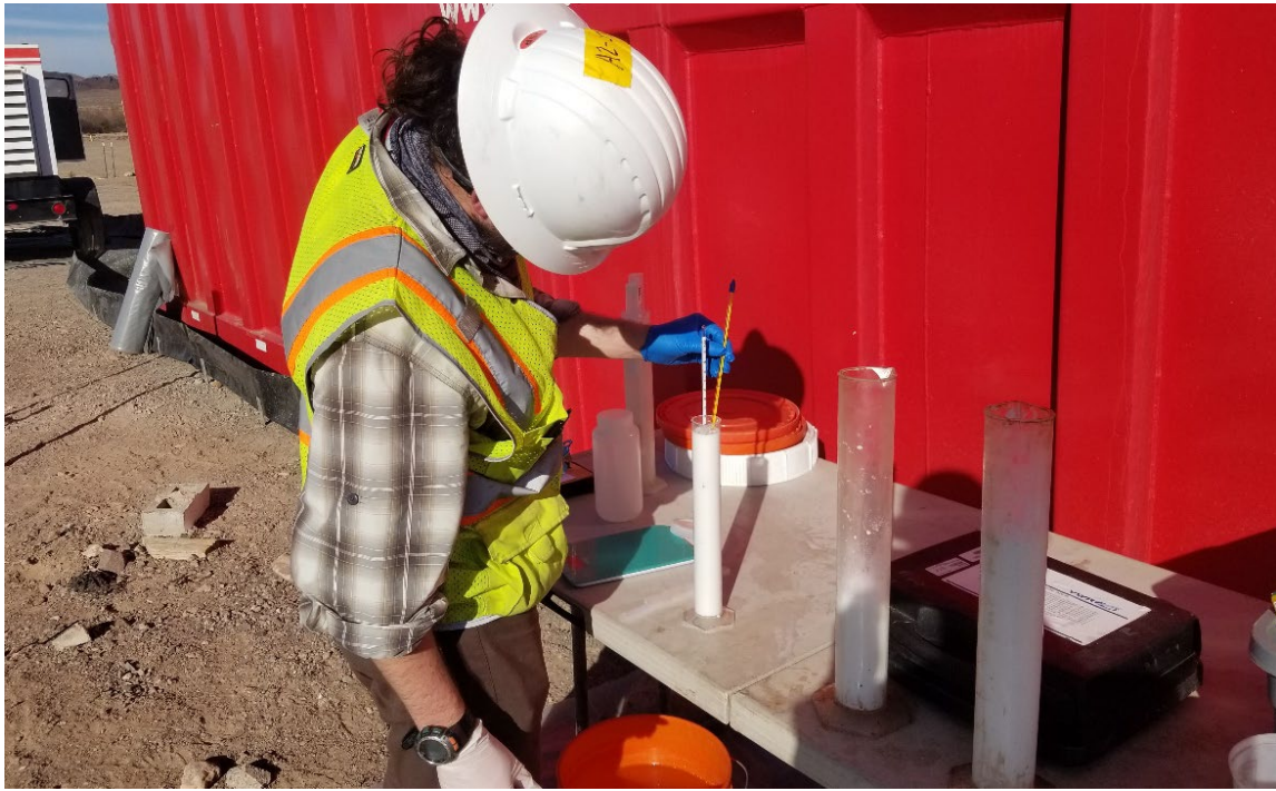
Collecting Temperature and Specific Gravity Measurements of Carbon Substrate Solution (EVO, Extracted Groundwater, and Amendments) to Confirm Batch is Properly Mixed Prior to Injection
