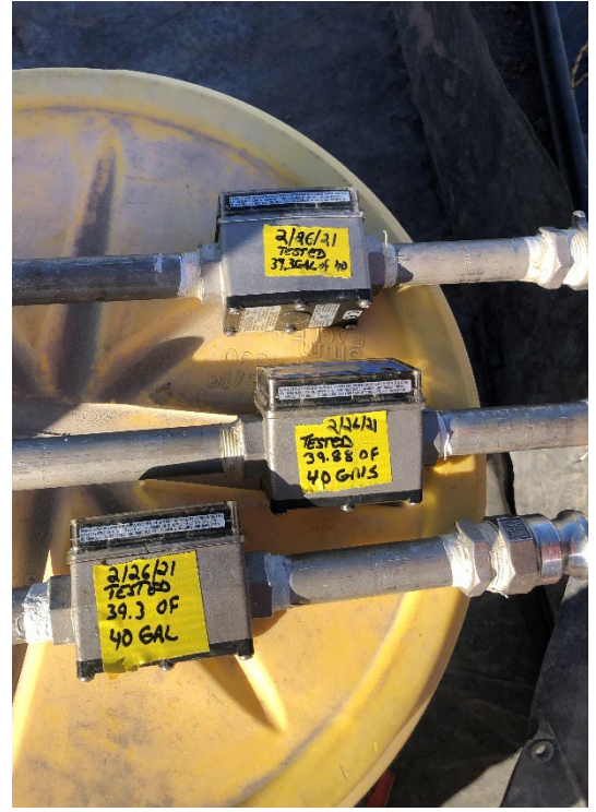
Left: Testing and calibrating flow meters; Right: Tested flow meters
