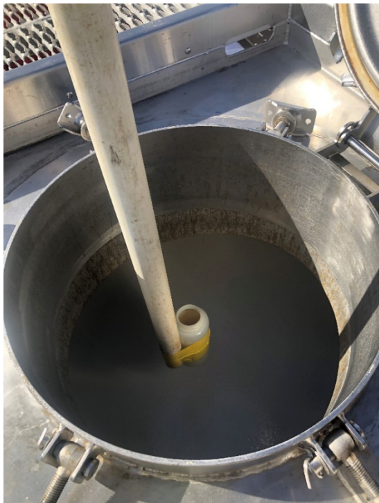
Left: Collecting EVO Sample from Tanker for Batch Standard Measurement; Right: Tank Level Measurement Setup to Confirm Batch Quantities during Batch Mixing
