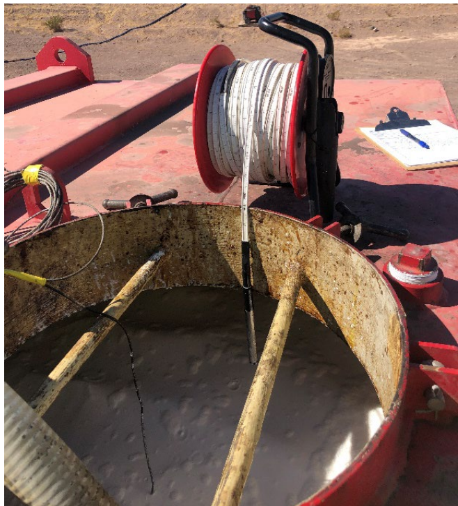
Left: Collecting EVO Sample from Tanker for Batch Standard Measurement; Right: Tank Level Measurement Setup to Confirm Batch Quantities during Batch Mixing
