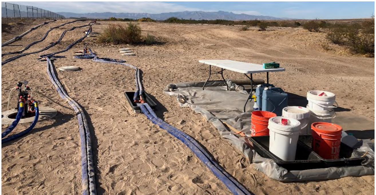
Dye study testing station to collect periodic samples from nearby dose response monitoring wells.
