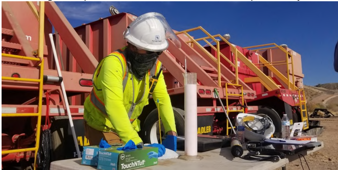
Measuring specific gravity in a batch sample using a hydrometer.
