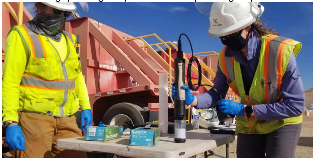
Measuring rhodamine dye concentrations in a batch sample using a field probe.
