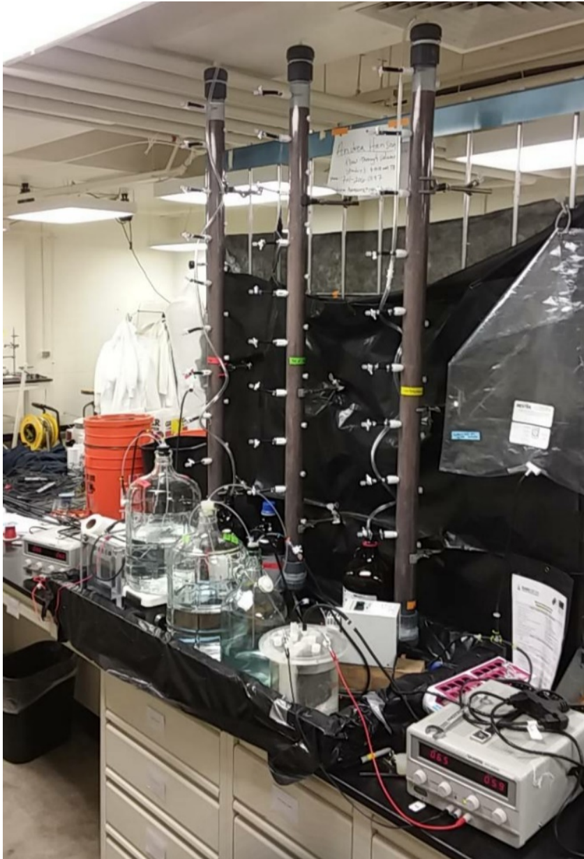
Photo 1. Flow-through column tests with site soils. Column test experiments from left to right: 1) indirectly treated groundwater (electrochemically generated hydrogen sparged as only electron donor); 2) untreated groundwater (no added electron donor); and 3) electrochemically treated groundwater (hydrogen and organics from cathodic reduction as electron donors).
