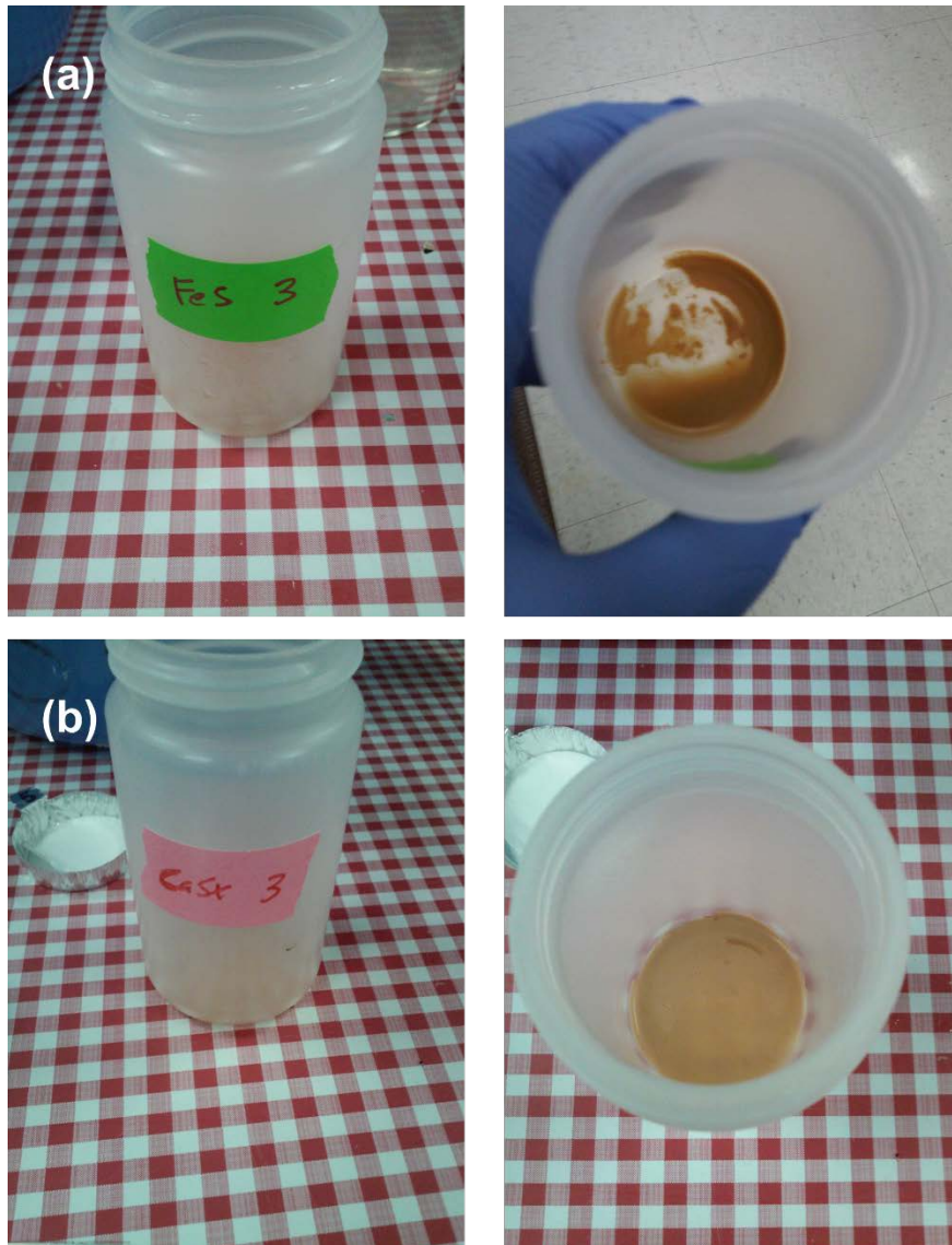
Figure F.5: Sludge content for low-range concentration for QAL groundwater 25 to 30 feet bgs) with 0.50 mg/L Cr (VI): (a) groundwater with ferrous sulfate and (b) with calcium polysulfide.
