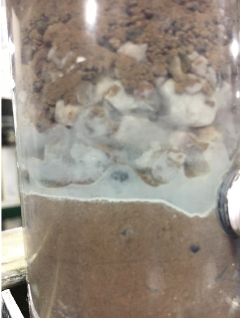
Figure F.10: Injection port on QAL column Day 16 shows the white scale formation at the injection port
