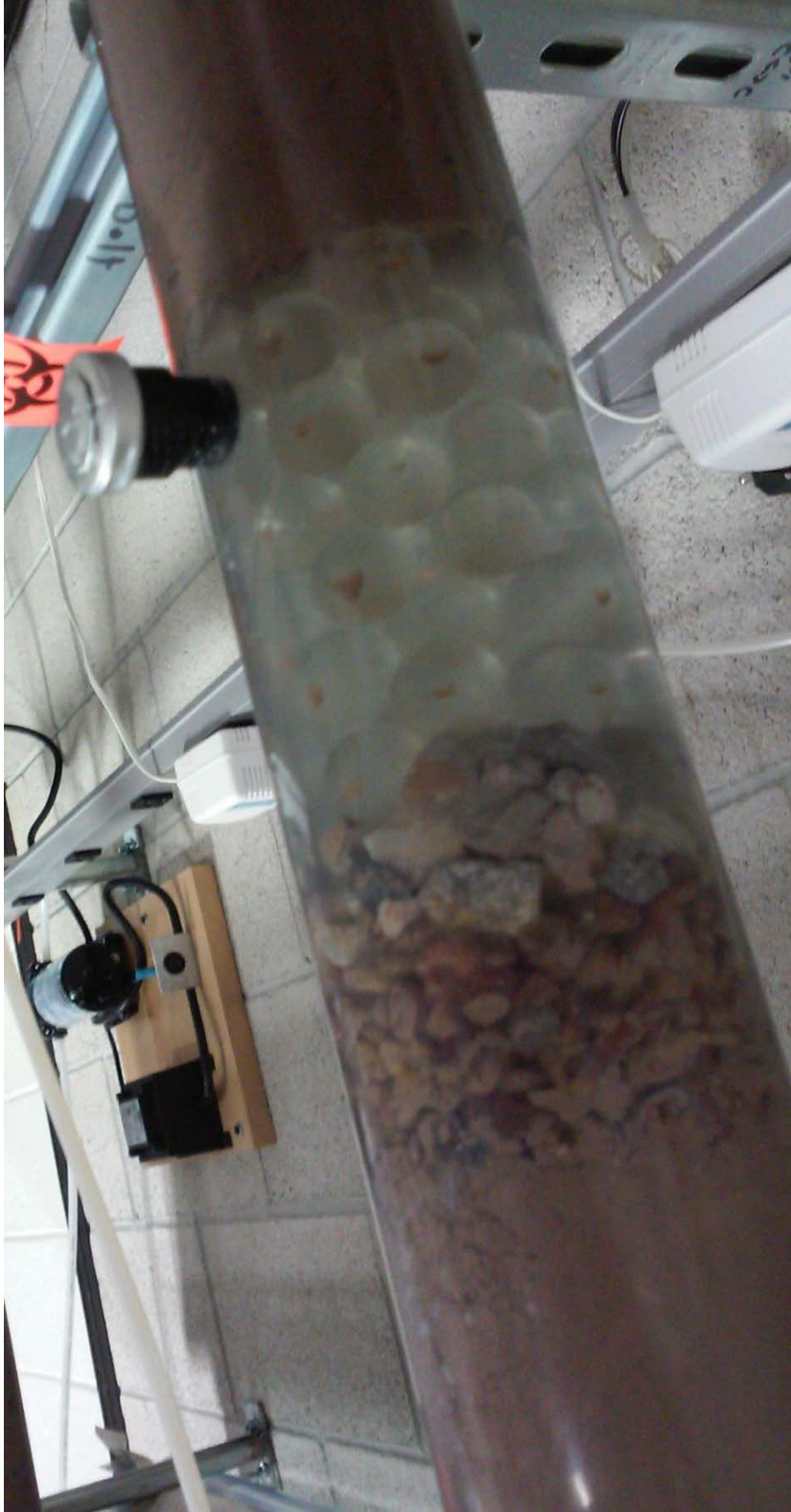
Figure F.12: Injection port showing with gravel and glass beads.
