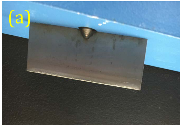
Figure F.6: Stirrers after operating batch precipitation test with groundwater from 25-30 ft containing high-range chromium concentration: (a) ferrous sulfate or (b) with calcium polysulfide showing that no inorganic scales were formed on the stirrer.
