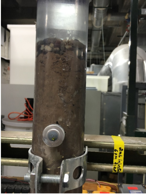
Figure F.8: Injection port on UMCf column Day 16
