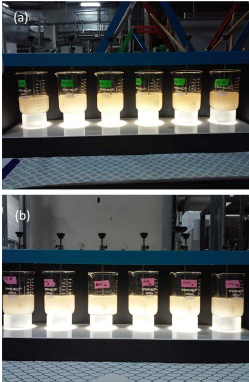
Figure F.3: Low-range concentration batch experimental set-up for QAL groundwater (25 -30 feet bgs) (a) groundwater with ferrous sulfate and (b) with calcium polysulfide.
