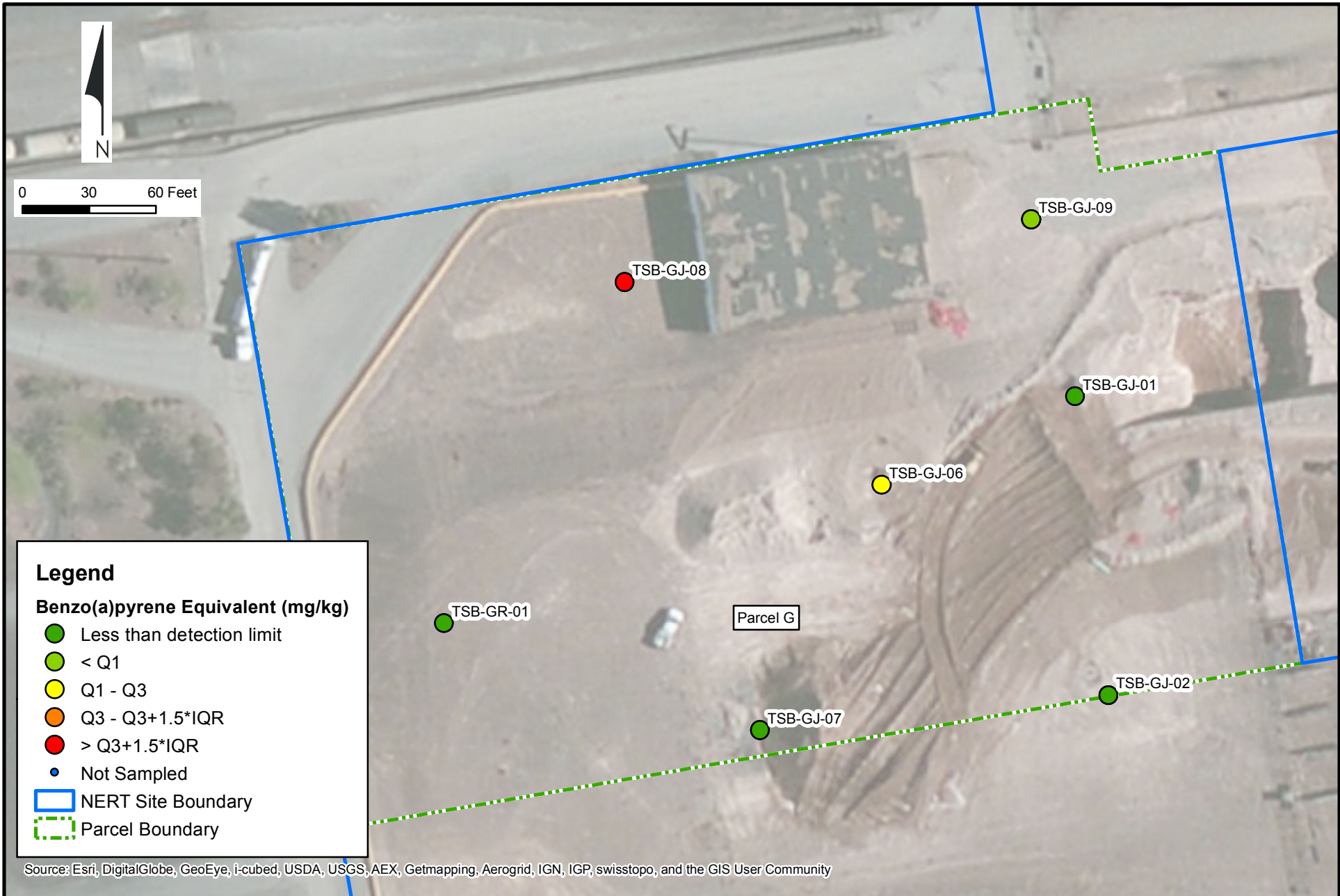
Spatial Quartile Plot for Parcel G - Benzo(a)pyrene Equivalent (mg/kg) [Q1 = 0.0212, Q3 = 0.0385, Q3+1.5*IQR = 0.0644] Nevada Environmental Response Trust Site; Henderson, Nevada
