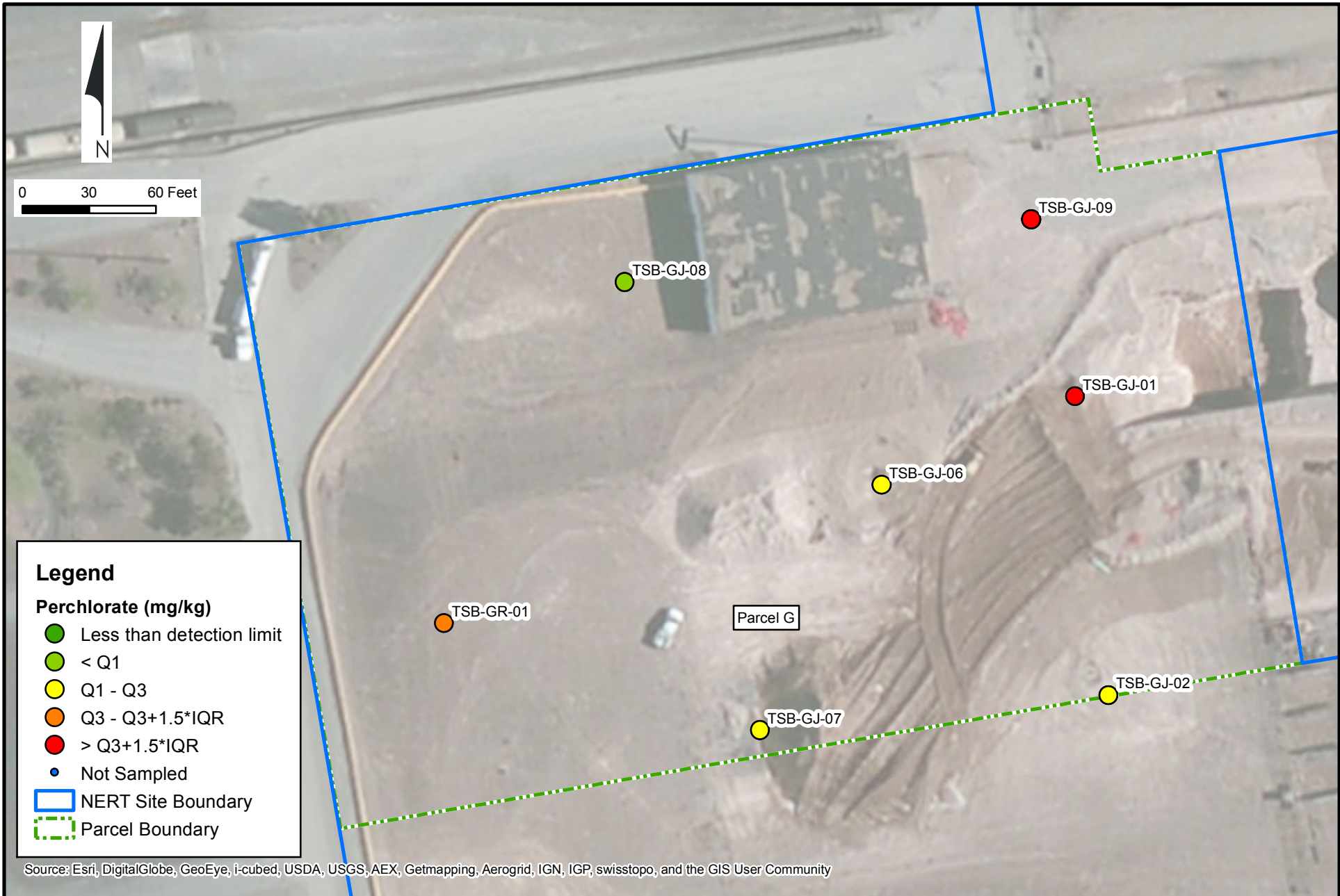
Spatial Quartile Plot for Parcel G - Perchlorate (mg/kg) [Q1 = 0.662, Q3 = 5.65, Q3+1.5*IQR = 13.1] Nevada Environmental Response Trust Site; Henderson, Nevada
