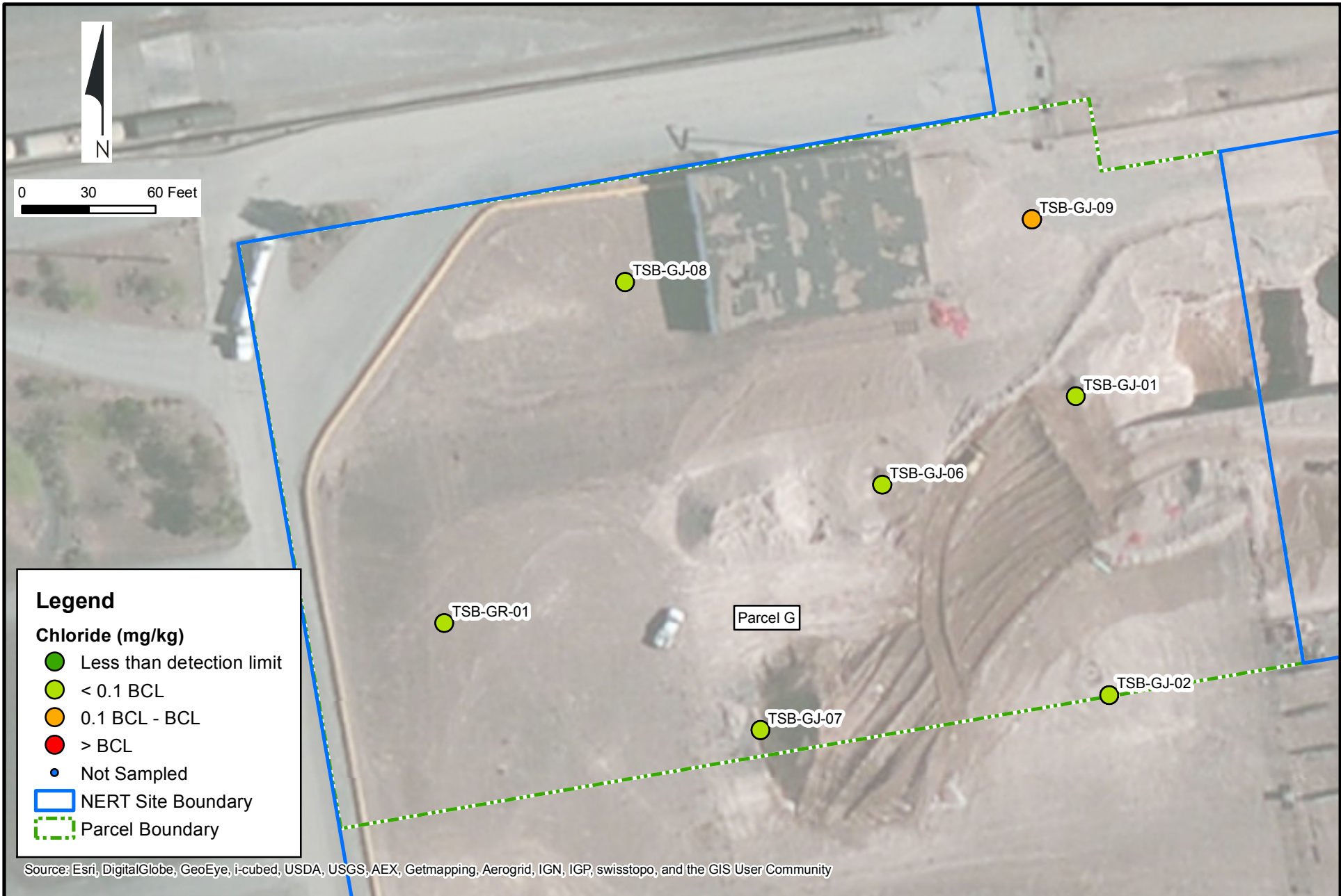
Spatial Intensity Plot for Parcel G - Chloride [BCL = 113032 mg/kg] Nevada Environmental Response Trust Site; Henderson, Nevada
