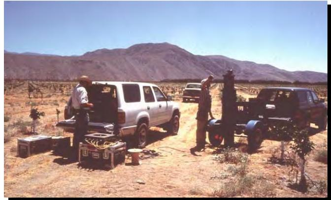
Seismic Refraction Survey in the Borrego Valley
