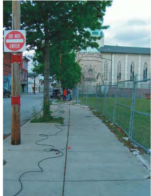
***Microtremor Measurements along Sidewalk***
