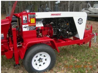
Injection pressures typically do not exceed a few hundred psi, but each site will impose its particular requirements. The volumetric rate should exceed 25 gpm for adequate process performance as well as cost-effective deployment.
