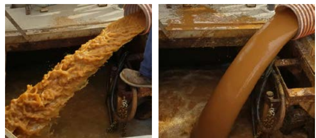
Effluent during pigging operations. Immediately before (left) and after (right) pig discharge.
