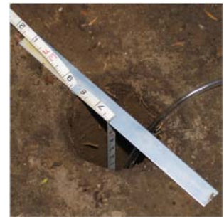
Fig. 19. Tape secured using Tape Holder.
