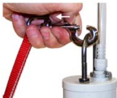
Fig. 15. Connecting Tape Hook to RU.
