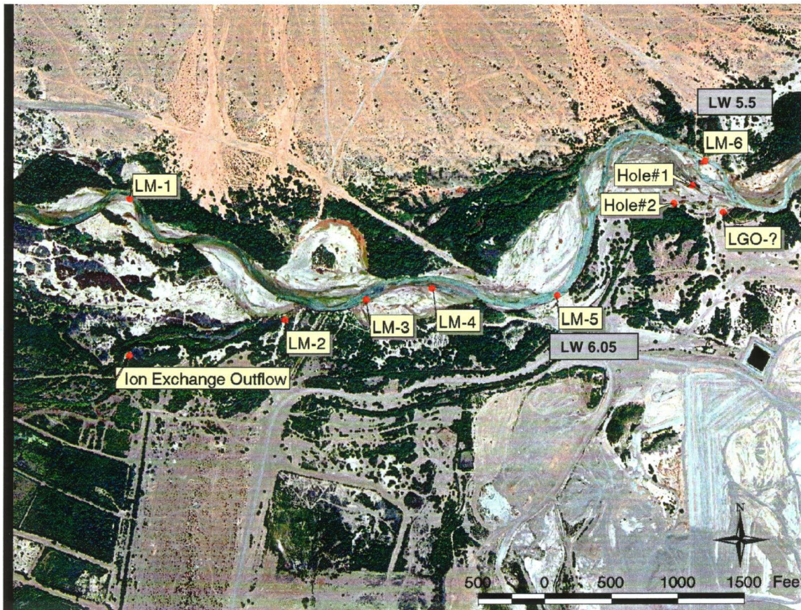
Figure 1 – Photograph of Las Vegas Wash study area. Dye will be injected at approximately LM-2 and transect fluorescence measurements will be made downstream toward LW 5.5 (formerly LM-6).
